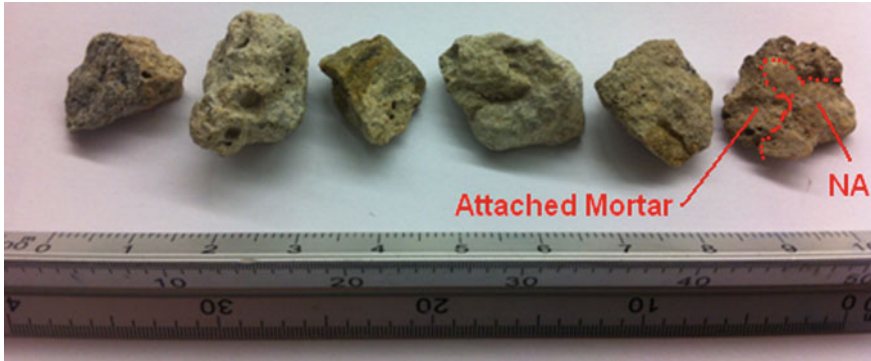
Fig. 3.12 Recycled aggregates with high attached mortar content
