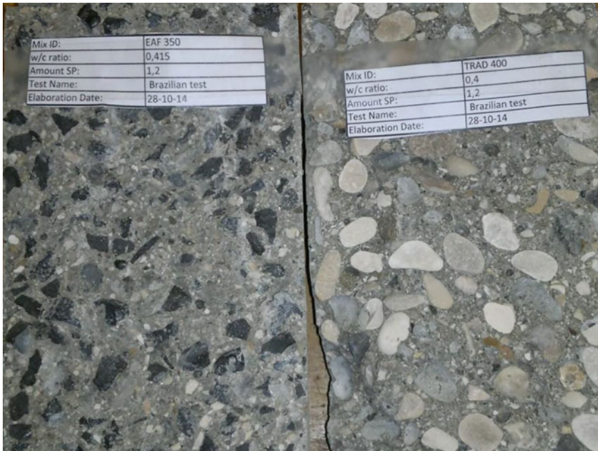
Fig. 4.19 Splitting failures of two HPC concretes
